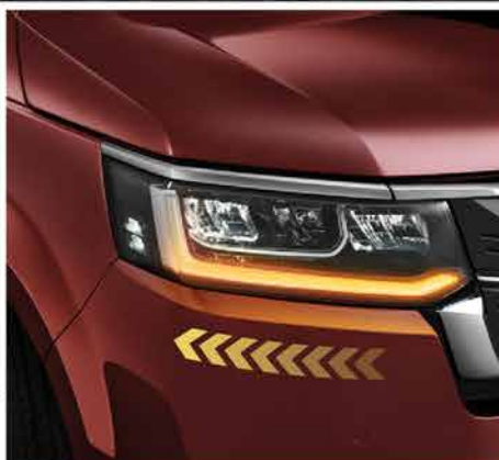
Sequential LED Turning Signal with Active Cornering Lights
