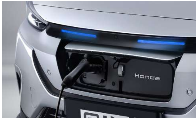
Charging Port with LED Indicator Lights (Support DC Fast Charging)
